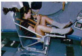
f / The time for one cycle of vibration is related to the object’s mass.
